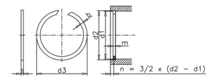
$\begin{array}{lll} b & = 3.40 \\ d1 & = 102 \\ d2 & = 104.3 \\ d3 & = 105.3 \\ Description = SB 102 \\ FN kN & = 62.00 \\ FR kN & = 53.60 \\ m min & = 2.7 \\ \end{array}$
